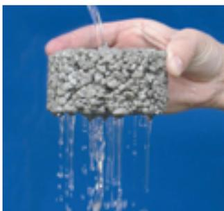
This is a special mixture of concrete that can be poured and leveled the same as conventional concrete. It can be used just about anywhere, including parking lots, roadways and sidewalks.
