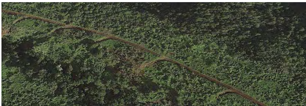
Figure 5: Aerial photograph showing dirt road and 'kickouts' which deliver road runoff and sediment into the gulch. The left side of picture leads downslope towards the ocean. Preliminary surveys identified 65 kickouts in Honokōwai Watershed and 55 in Wahikuli Watershed actively contributing sediment to adjacent streams.
