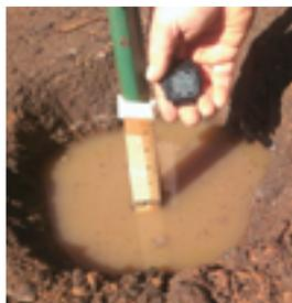
**Illustrative example:** If the water level dropped by 5 inches over 4 hours, divide 5 by 4, which equals 1.25, giving you an infiltration rate of 1.25 inches per hour.
